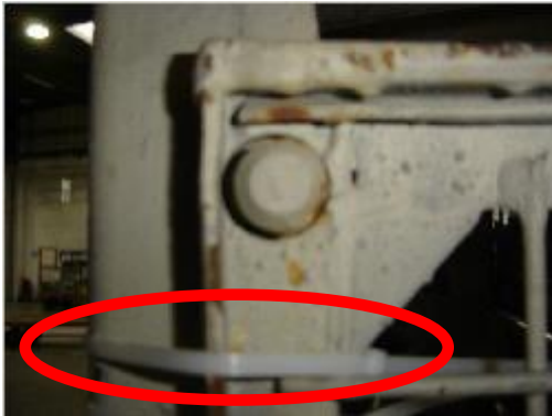
Exchangeable: Cable tie is serving the additional securing
